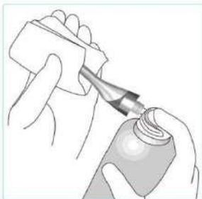
Screw the nozzle onto the spray can. Then insert it into the connection end of the contra-angle, and spray for 2s-3s. Using gauze to wipe off the excess oil from the outside of the contra-angle.
