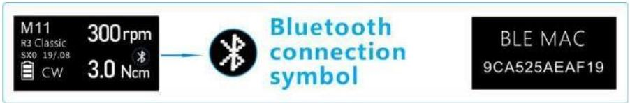
Meanwhile, the advanced mode setting also provides the MAC address of the Bluetooth function of the instrument. It is convenient for other devices to identify the Bluetooth address when searching the Bluetooth connection of the instrument.
